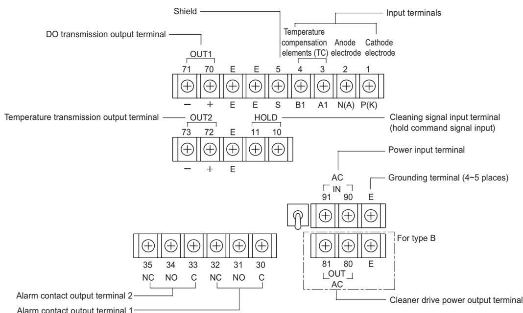
**Type C and D (2-point alarm contact output with a power cut-off signal output terminal)**
