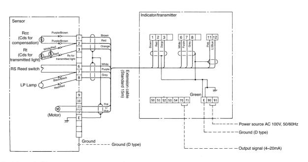
Terminal screw, size: M4 (Sensor ground terminal along: M5)
