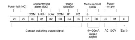
Contact switching input signal --- Contact Rating: DC 30V 0.1A
