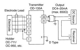
\* Optional feature: remote input to terminals 90, 11 for input "hold". <Use of junction box an extension cable>
