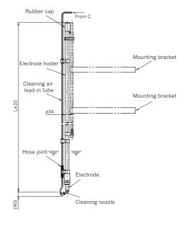
Pole stand Ø Rubber stopp 10 Control €00 80 unit 60.39 Mounting 100 40+ ∕bracket 4 10 8 Ø60.5 300±10 500 8 30± Protection Mounting bracket pipe 200 ~ 300 / Drop∙in type Cleaning air lead-in tube DO detecto 100 L=2~6m
